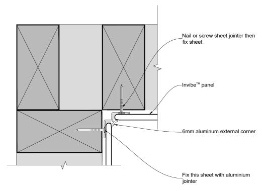
**Note:** All site cut edges to be sealed Silicone required in wet areas with Invibe™ panel
